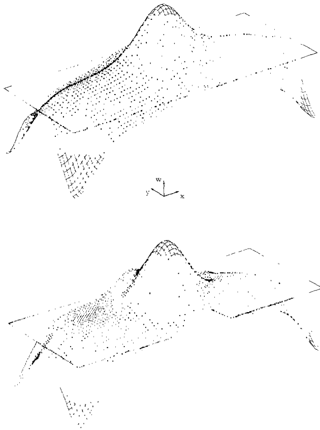
FIG. 1. Vertical velocity at the midlayer for P = \infty (top) and P = 20 (bottom), with R = 40,000 , a = 2.5 , and b = 6 .
